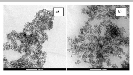
Fig. 1: TEM Images a) Magnetic Iron Nanoparticles (MNPs) b) Chitosan coated MNPs (CNPs)
