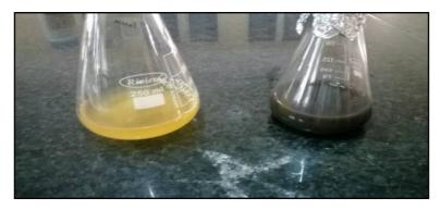
Fig. 1.Synthesis of silver nanoparticles from leaf extract incubated with silver nitrate solution
