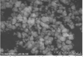
Fig.3. FESEM image of silver nanoparticles synthesized using P.latifolia leaves
