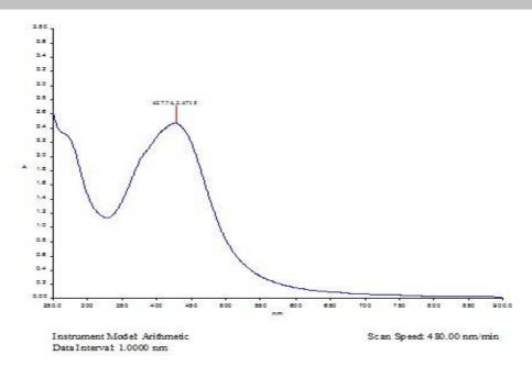
Fig: 1 UV-VIS spectroscopy of silver nanoparticles synthesized using B.magnifica leaves.
